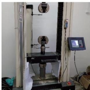
图5  $\phi 100 \text{ mm} \times 200 \text{ mm}$  试块单轴压缩试验Fig.5 Uniaxial compression test of  $\phi 100 \text{ mm} \times 200 \text{ mm}$  specimen
